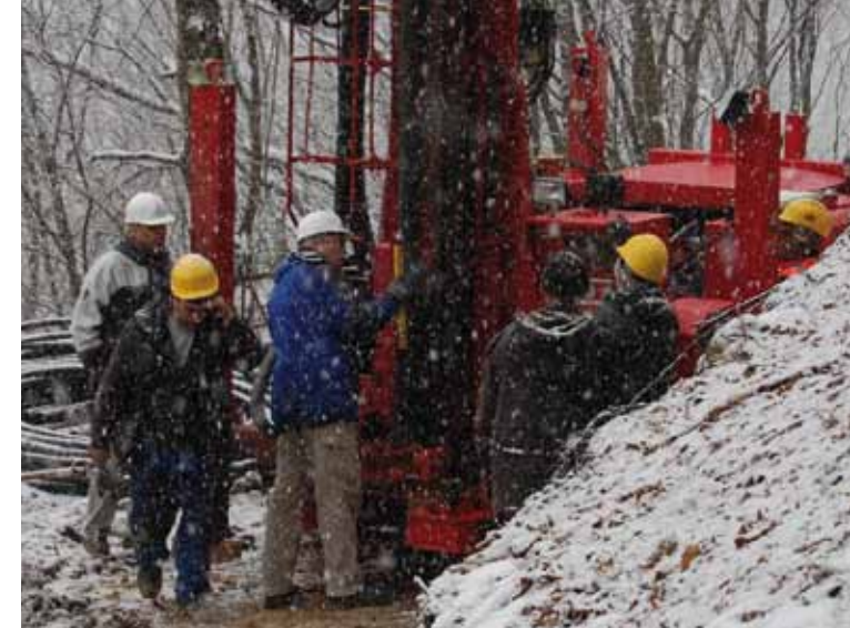
The drilling set up for our first of 3 one thousand metre holes in Romania from this past February.
